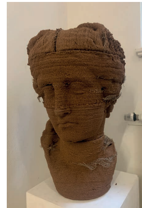
Thermoplastic cork- gelatin compound for 3D printing, research project "GreTA" / recyclable base structures for theat- rical sculpture using nature-based raw materials
